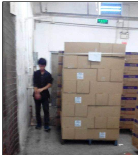
Blocked emergency exit
