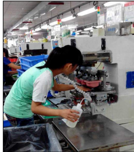
A worker cleaning devices using thinner without wearing protective mask and gloves.
